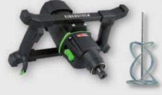
EHR 23/2.5 S Set 1.800 W; 0-250/0-580 min -1 ; Ø 180 mm; Rührgutmenge 80 kg
