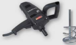
EHR 14.1 SK Set 960 W; 0-390 min -1 ; Ø 120 mm; Rührgutmenge 30 kg
