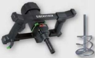
EHR 18.1 S Set 1.100 W; 0-450 min -1 ; Ø 120 mm; Rührgutmenge 40 kg
