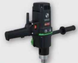
EHB 32/2.2 R R/L 1.800 W; 60-140/200-470 min -1 ; Ø 32 mm in Stahl
