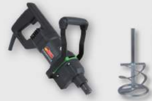
EHR 15.1 SB Set 1.050 W; 0-450 min -1 ; Ø 120 mm; Rührgutmenge 40 kg
